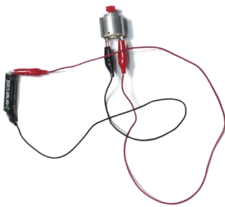
Motor connected to a single battery
