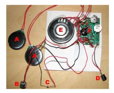
**Step 3 – Recording:** Press the two record buttons labeled "A" together until they click and the LED labeled "C" lights up. This indicates the module is recording. Speak into the microphone labeled "B". You will have 13 seconds of record time.
