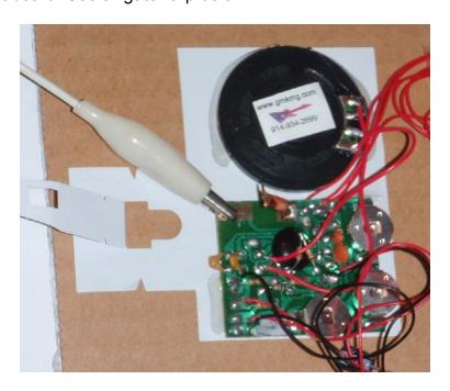
**Step 6:** Connect another wire with an alligator clip to the metal tab you pulled up from the board in step 4.
