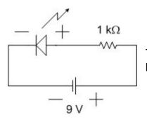
This circuit diagram is called a **schematic** and shows a 9 V battery in series with a 1 k $\Omega$  (1000 $\Omega$ ) resistor and an LED.
