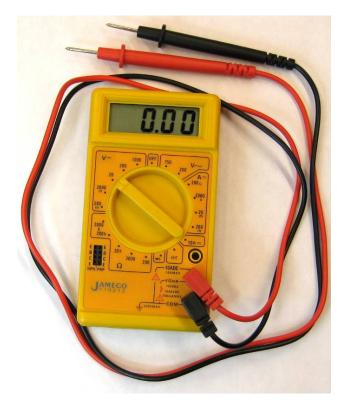
Set the dial on the front of the multimeter to 20 V DC (DC means constant). You do this by rotating the dial until the indicator points to 20 V DC as shown in the picture to the left.
