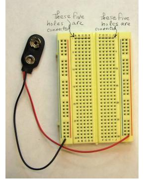
The **terminal strip is used to connect components** such as resistors and LEDs.
