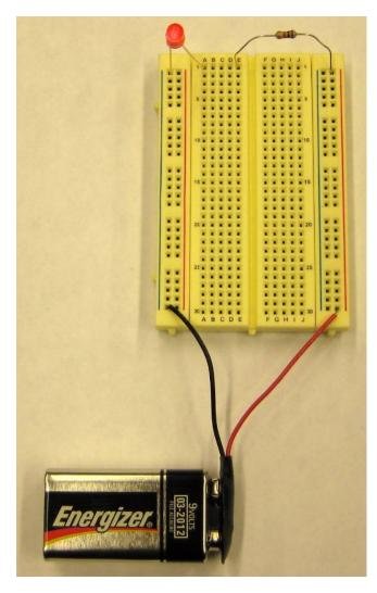
Obtain a 1 k $\Omega$  (1000 $\Omega$ ) resistor (brown, black, red) and a red LED. Build the circuit by plugging these elements into your breadboard as shown in the picture. Remember that the **longer lead** of the **LED** is **positive (+)** and the **shorter lead** is **negative (-)**.
