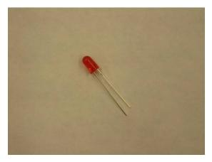
Picture of an **LED** The longer lead is positive (+) and the shorter lead is negative (-).
