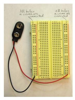
The **bus strips** are used for **power supply rails**.
