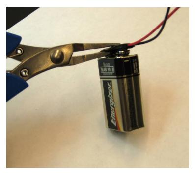
Remove the battery snap from your battery. You may need to use the needle nose pliers to remove the battery snap.
